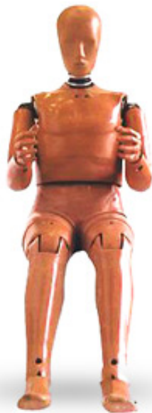
Hybrid III: designed to gather data from frontal impacts
