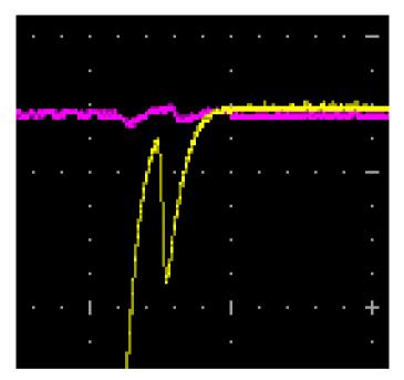
With CLK=1MHZ, glitch 50ns after the edge, pulse is 20ns wide. Works each time : <u>skip an instruction</u>.
